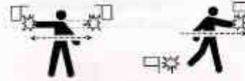
Horizontal waving of white flag, light or flare. Putting red flag, light or flare on ground and moving off with a second indicates direction of safer landing.
